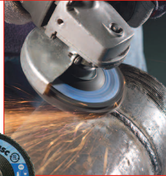
Blending a weld on the outside diameter of steel piping.
