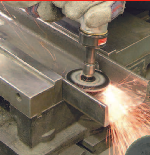
Tight area surface blending with a BobCat disc.
