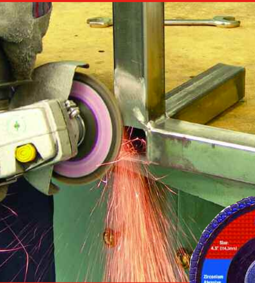
Grinding welds on a fabricated steel part.
